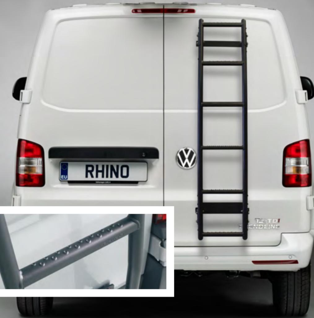
The Rear Door Ladder has been designed to blend aesthetically with the van styling and has user-friendly round hand rails and anti-slip plates to enhance safety.
